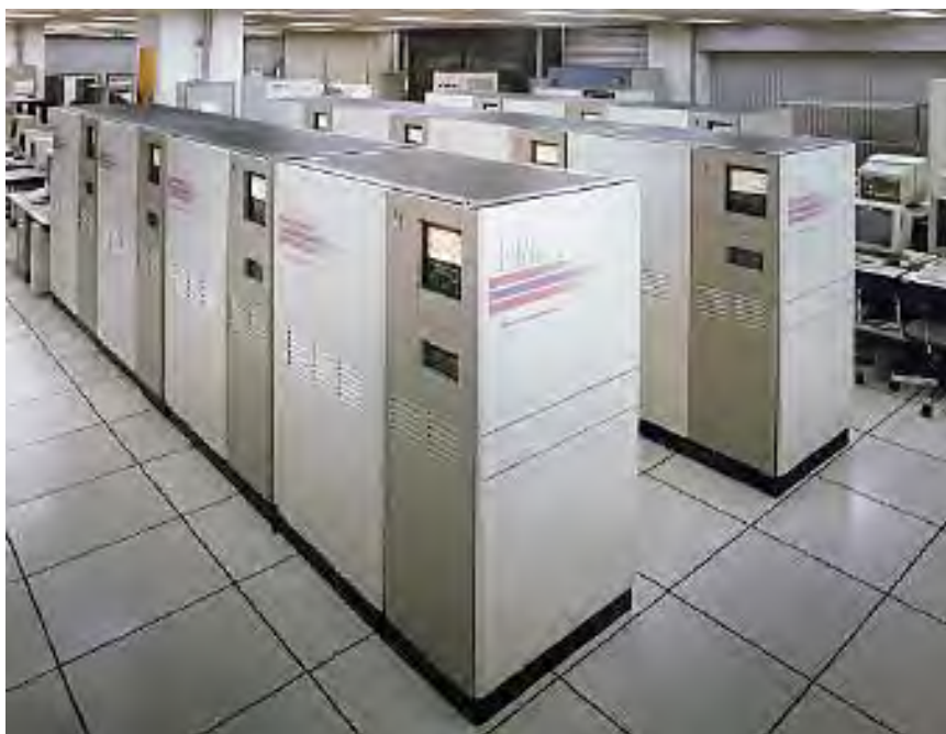
Figure 22.3: The PIM/p parallel computer system. (Photograph from http://www.icot.or.jp/ARCHIVE/Museum/MACHINE/pim-spec-E.html .)
